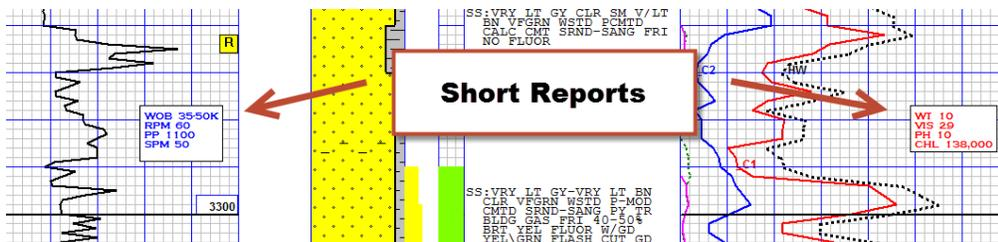
You can have more than one short report at the same depth, provided the locations allow them to be displayed without interfering with each other. The Short reports can be turned on and off in SETUP...LINES AND SCALES, by checking or un-checking Hide Short Reports.
