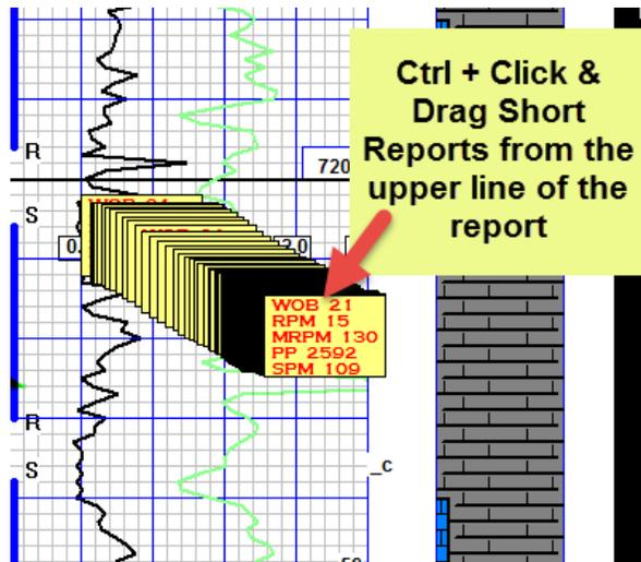
If the Drilling Report and the Mud Report are both selected to be viewed from the same short report, then the mud report will be controlled vertically on the log by movement upward or downward of the drilling report. The mud report can only be moved horizontally in this scenario.
