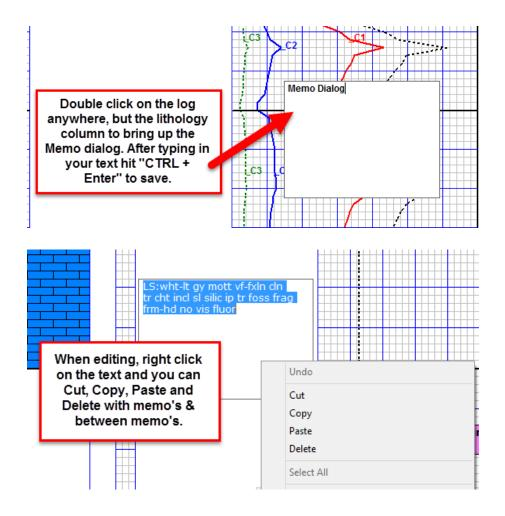
The second way to create a memo on the vertical log is **"CTRL+ left click & drag"**, down and to the right on the log. You can size the dialog by the direction of how far you click & drag, then type in your text and <u>"Ctrl + Enter"</u> to save. Each memo is limited to 500 characters on the Vertical log and the Horizontal Log.
